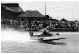
Initially the Warren. inboard boats had engines, often marinised car engines: gradually outboards made an appearance. The 'planes' themselves were manufactured Ωf plywood in sheds and
